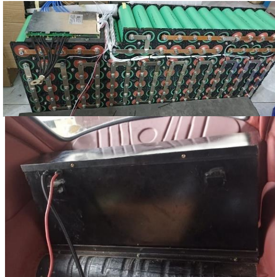
Gambar 8 bank B battery pack (bagian belakang)
